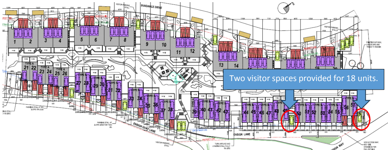
Figure 4: Visitor parking spaces not proportional to number of units and prohibitive to those with mobility challenges.
