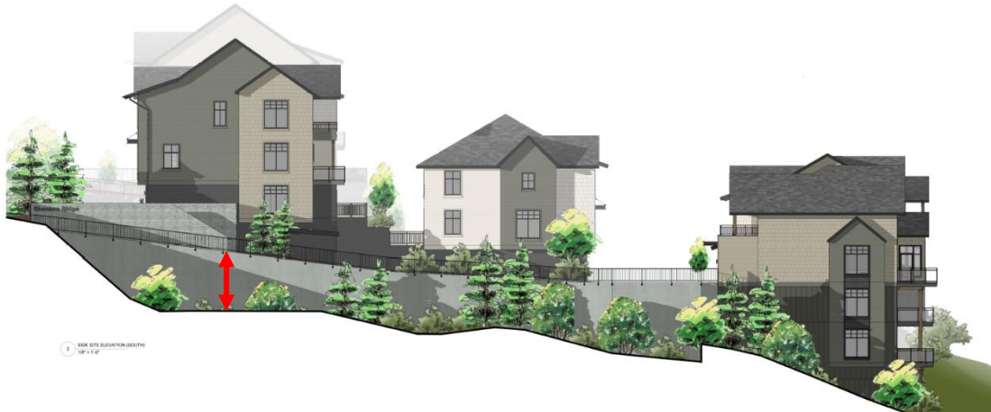
Figure 5 – Highest retaining wall adjacent to interior side parcel boundary. Wall will be screened by landscaping in front of the wall and a self-clinging vine on the wall itself.
