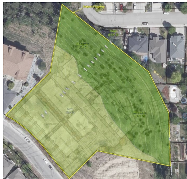
Figure 4 – Proposed development overlaid on environmentally sensitive areas and contour line mapping. Majority of development proposed within Environmental Sensitivity Area (ESA) 3 – Low (light green) and in flatter portion of the site.
