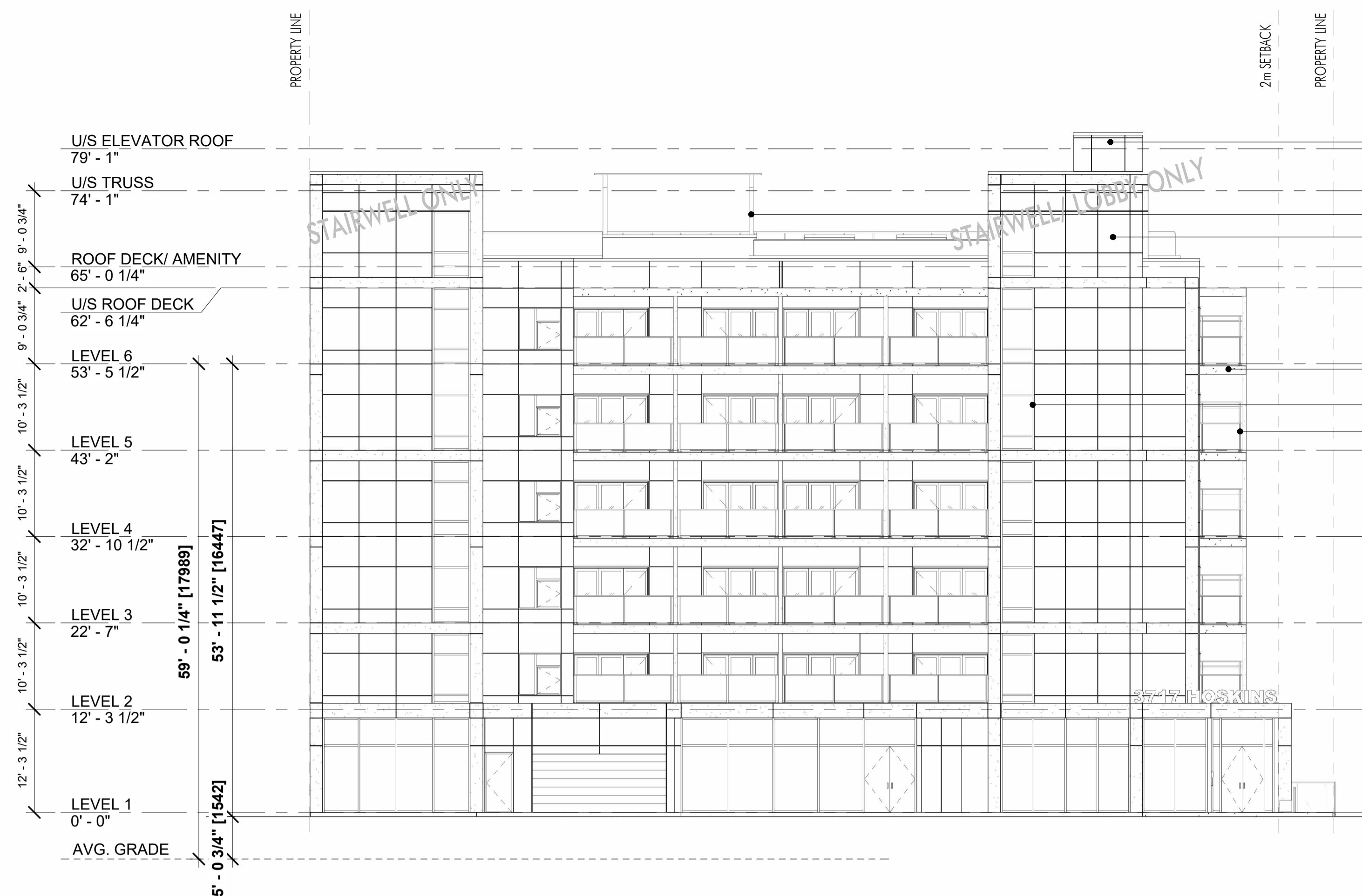
1 WEST ELEVATION (VIEWED FROM HOSKINS ROAD) A-200 3/32" = 1'-0"
