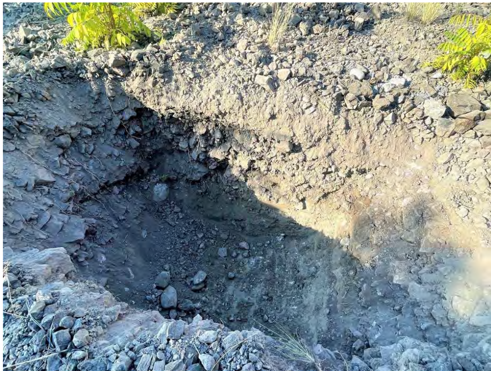
Photo 04 Test pit TP23-02 excavated profile
