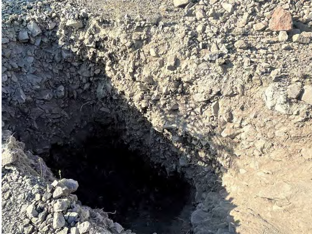
Photo 03 Test pit TP23-01 excavated profile
