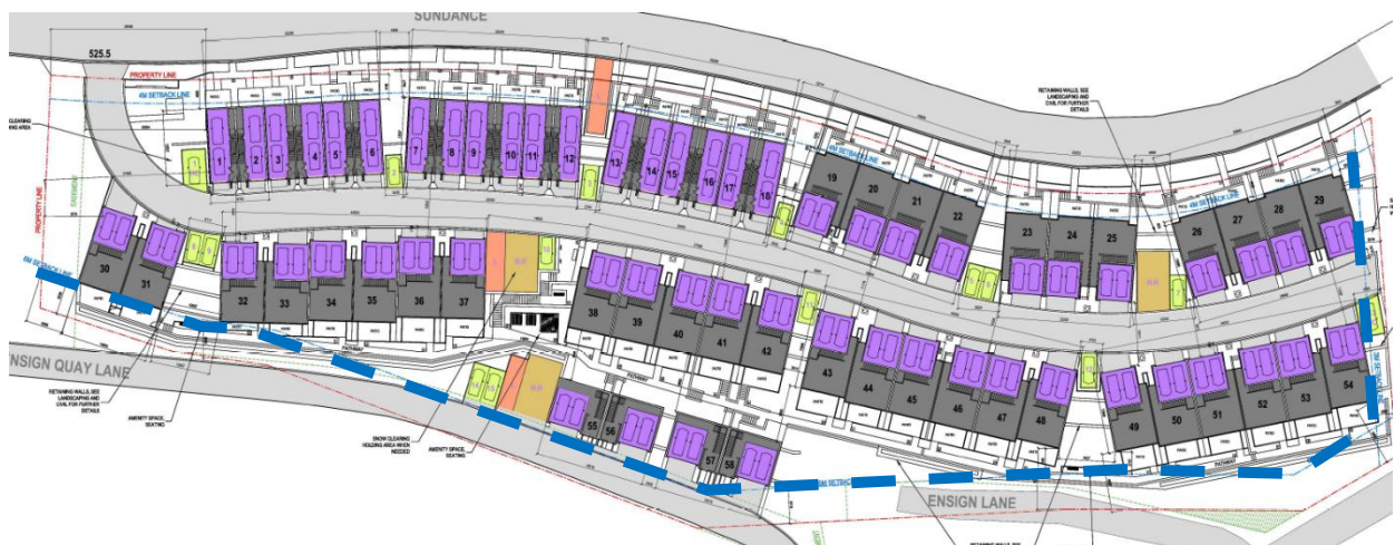
Figure 10: Markup of site plan showing impact of rear yard and interior side boundary reductions (blue dashed line)
