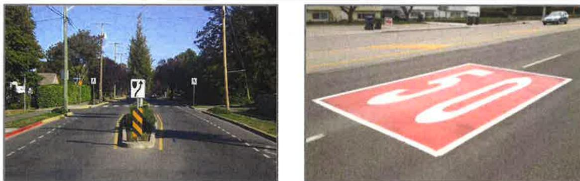
Figure 4: Landscaped Median (Left) and 50km/h Pavement Marking (Right)
