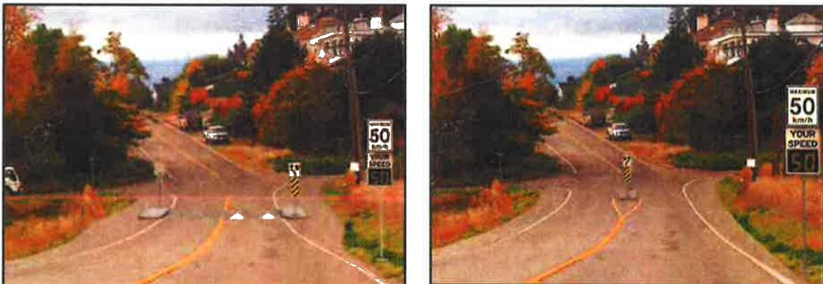
**Figure 2: ISL Proposed Gateway Treatments with Speed Hump (Left) and Median (Right)**
