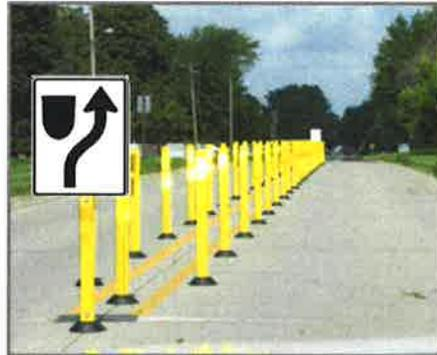
**Figure 5: Vertical Centreline Treatment with Flexible Delineator Posts**
