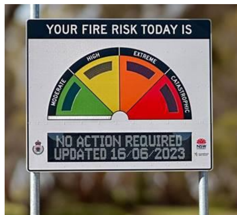
Example of electronic Fire Danger Rating sign.
