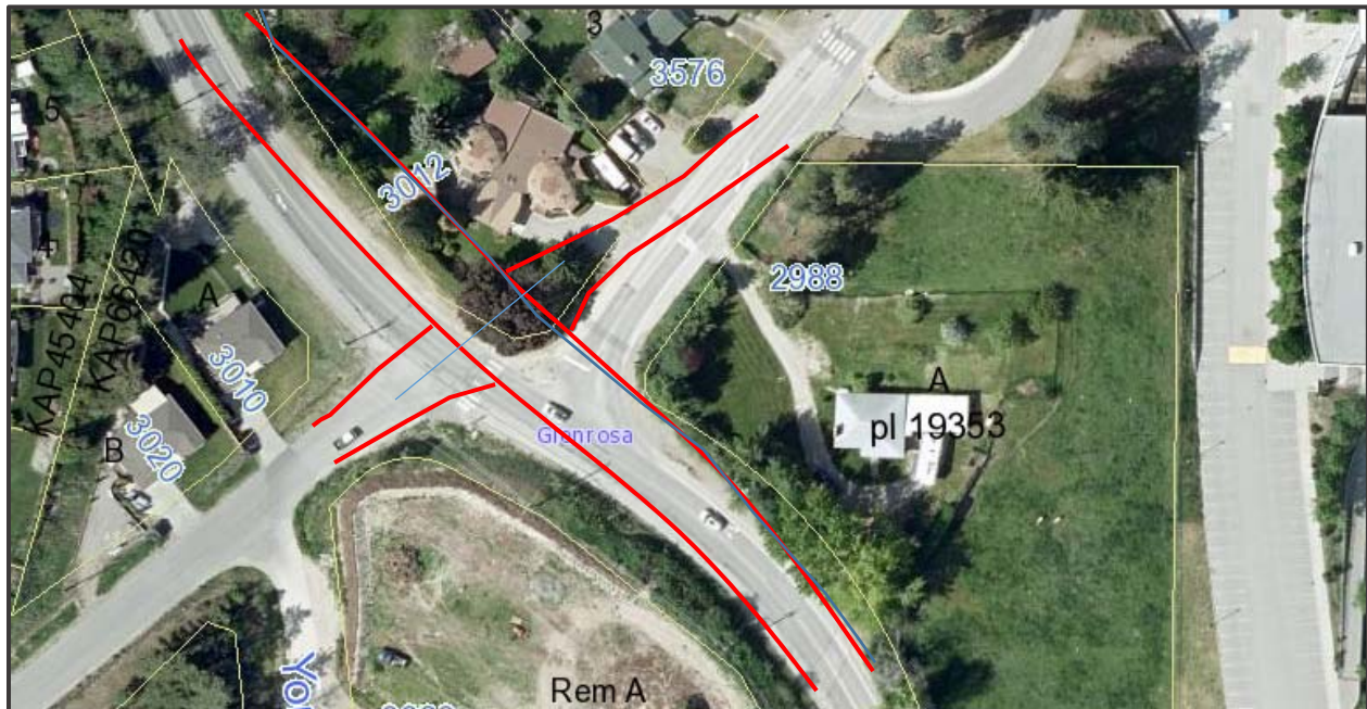
Figure 8: Sketch of Glenrosa Road and McIver Road East Leg Realignment
