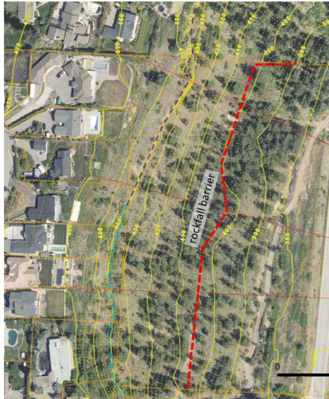
Figure 8: Conceptual Rockfall Barrier Location
